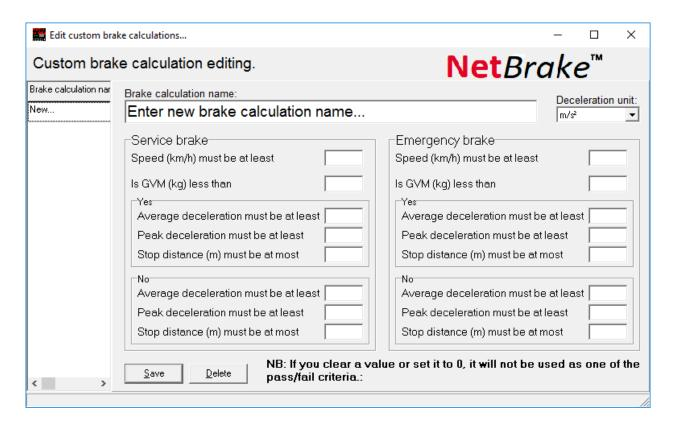
Deceleration unit. AutoStop Heavy brake testers are able to store average and peak deceleration in one of three units. Choose a preferred unit of measure here, and all deceleration values will be displayed in this unit for all vehicles associated with this brake calculation.
